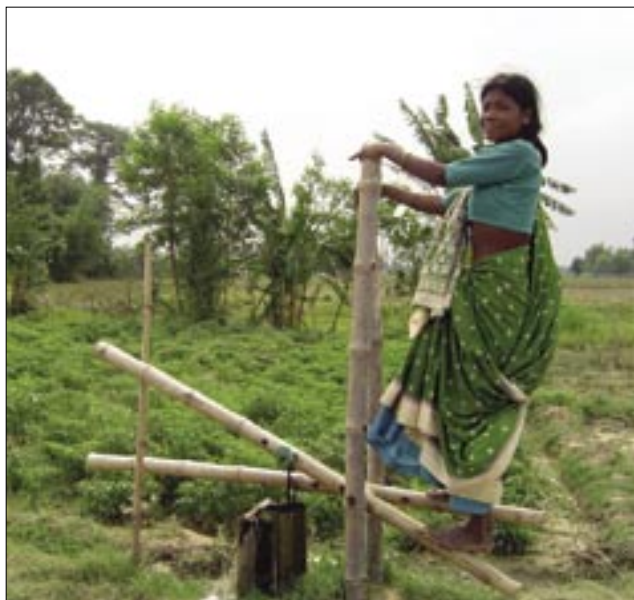
A woman operates a bamboo treadle pump in Nepal.
